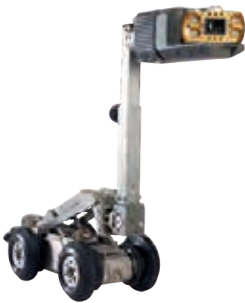
Height extension For centered camera position in larger diameters.
